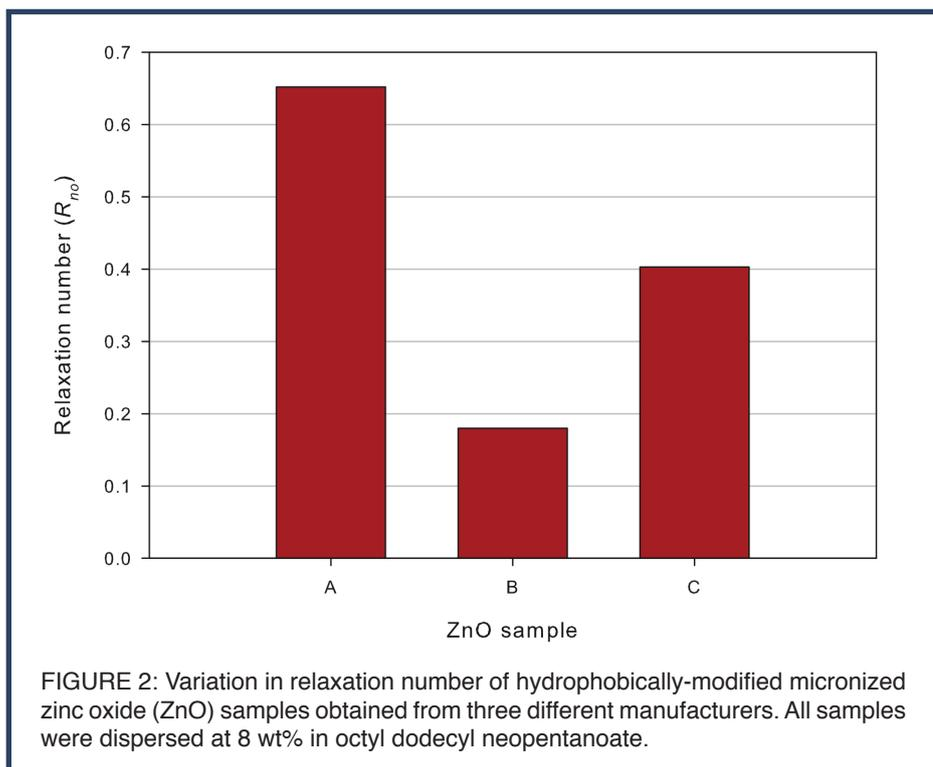
This case study demonstrates well how NMR relaxation data can be used not only for fast determination of powder wettability by liquids, but also to discriminate materials based (via coatings) on their surface chemistry and, by extension, how the *MagnoMeter* XRS™ can be used to select an appropriate dispersal fluid. This can aid in understanding how to develop and create improved suspensions which, in
