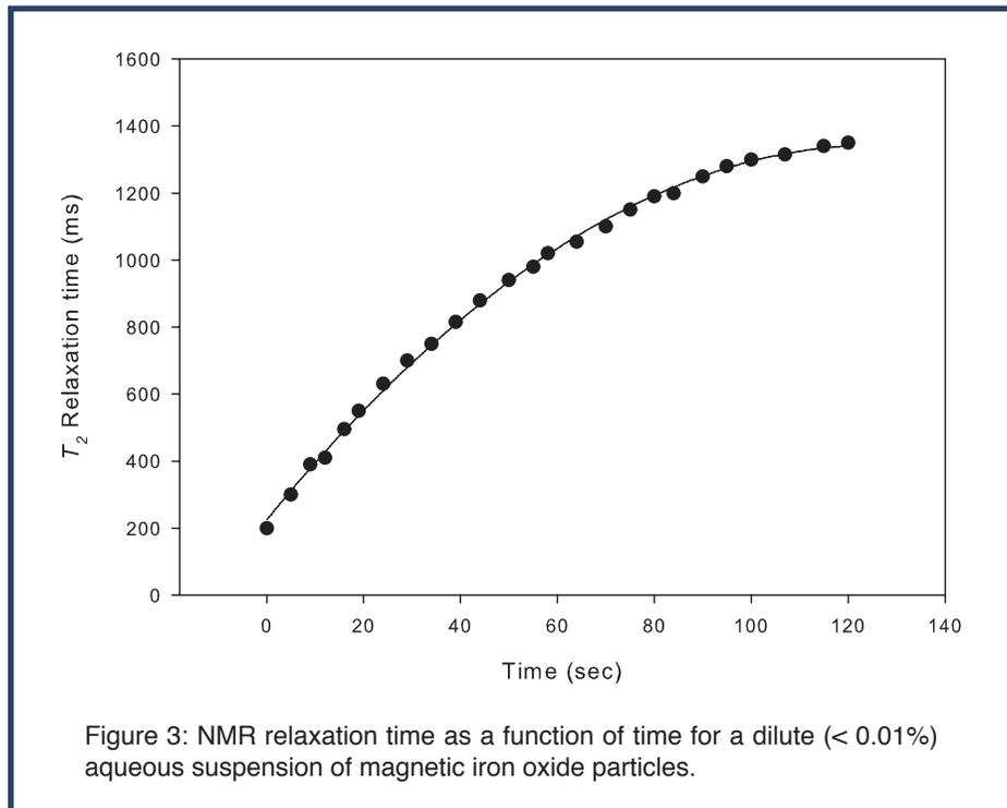
Hence, the *MagnoMeter XRS™* can be used to study not just sedimentation and settling but also kinetic processes, such as coagulation and flocculation (see Mageleka Application Note 16).
