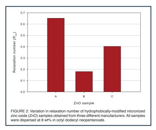
This case study demonstrates well how NMR relaxation data can be used not only for fast determination of powder wettability by liquids, but also to discriminate materials based (via coatings) on their surface chemistry and, by extension, how the *M*agno*M*eter XRS<sup>™</sup> can be used to select an appropriate dispersal fluid. This can aid in understanding how to develop and create improved suspensions which, in
