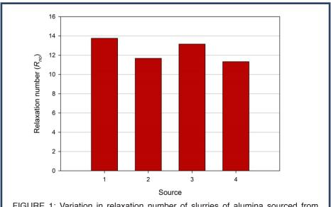
FIGURE 1: Variation in relaxation number of slurries of alumina sourced from different countries. All slurries were prepared at 37.5 wt% in ethanol.
