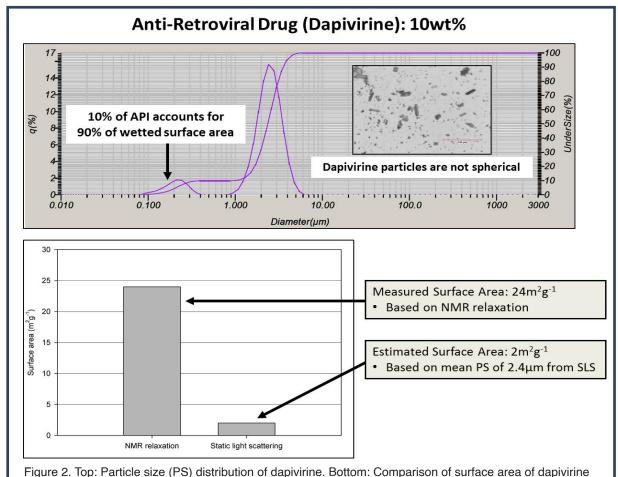
Particle size (PS) distribution of dapivirine. Bottom: Comparison of surface area of dapivirine particles measured directly by nuclear magnetic resonance (NMR) relaxation and estimated from mean particle size (PS) data derived from static light scattering (SLS).
