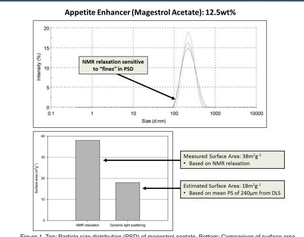
Figure 1. Top: Particle size distribution (PSD) of magestrol acetate. Bottom: Comparison of surface area of magestrol acetate particles measured directly by nuclear magnetic resonance (NMR) relaxation and estimated from mean particle size (PS) data derived from dynamic light scattering (DLS).
