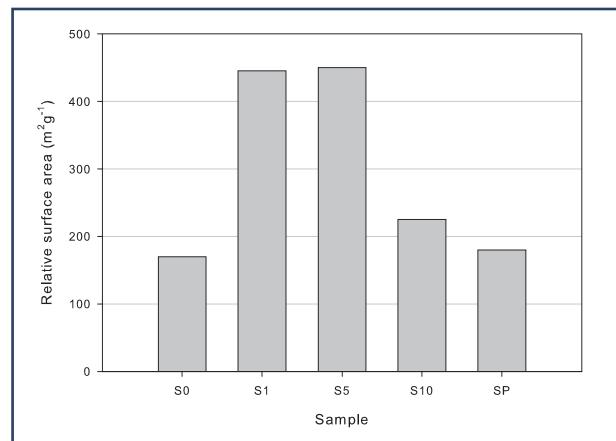
Figure 1. Wetted surface area, calculated from nuclear magnetic resonance relaxation time values (average repeatability <1.0% for all samples), of a series of samples of graphene powder dispersed at 2 wt% using a polymeric surfactant/dispersant at concentrations of 0%, 1%, 5%, and 10%. The "SP" sample was prepared at 20 wt% using production dimension equipment, but with no surfactant and gave similar results to S0.
